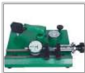
inspect accuracy of dial indicators (range 0-25mm)
