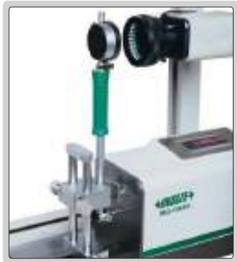
check bore gages
