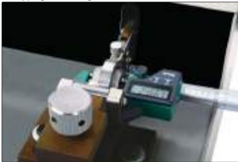
lapping measuring surfaces of outside micrometer
