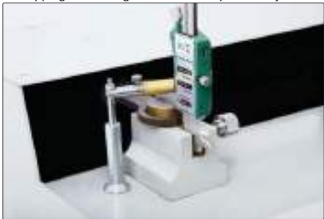
lapping measuring surfaces of caliper lower jaws
