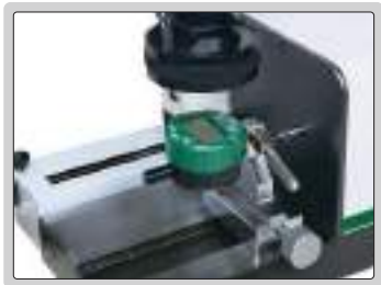
check digital indicators (detect digits on screen)
